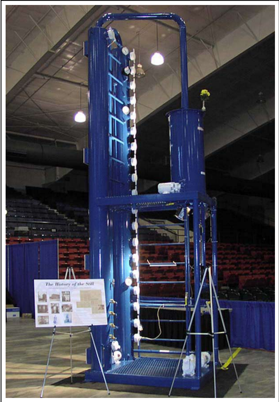
Figure 1. Distillation column of the SDSU farm-scale ethanol plant.
