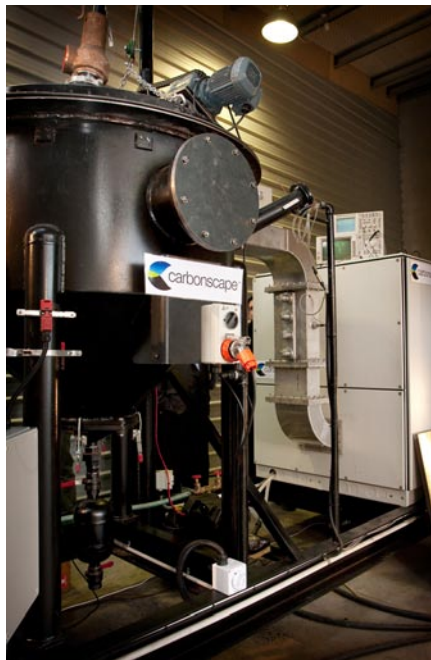
New Zealand start-up Carbonscape is using industrial-scale microwaves to turn biomass into biochar.
